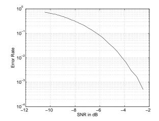
Fig. 6. Error rate versus signal-to-noise ratio - compressed images.
